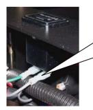
Hour meter has a **positive** and a **negative** post. Gray wire should go on the positive. Power is supplied from the ignition switch.
